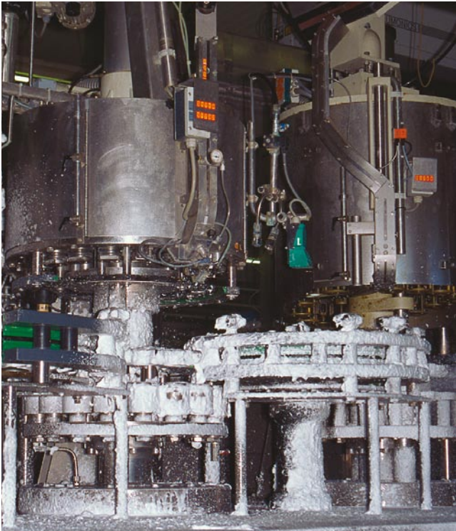
Beverage bottling systems in breweries are cleaned using aggressive media, which could destroy standard clutches without corrosion protection within a short period of time.
