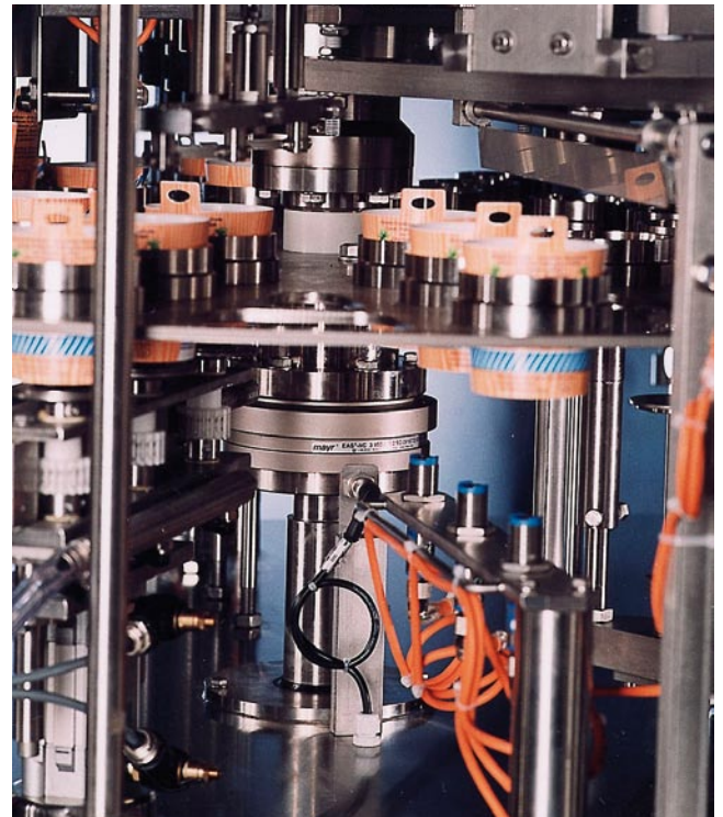
EAS®-Compact® rustproof with contactless limit switch in a filling machine for cream cheese.
